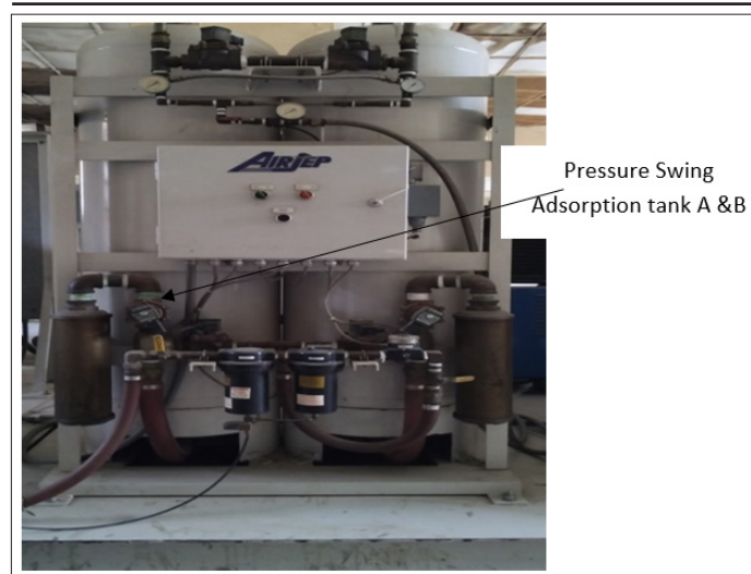
Figure 3: PSA Tank A & B
