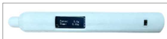
Figure 11: Completed Exterior Design of the Pressure-Sensing Massage Stick
