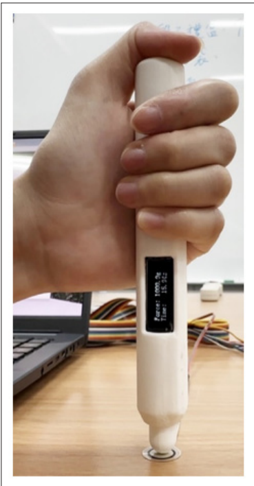
Figure 17: The Massage Stick was Tested Under an Applied Pressure of 1000 g
