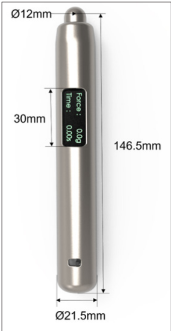
Figure 16: Finalized form Factor of the Pressure-Sensing Massage Stick
