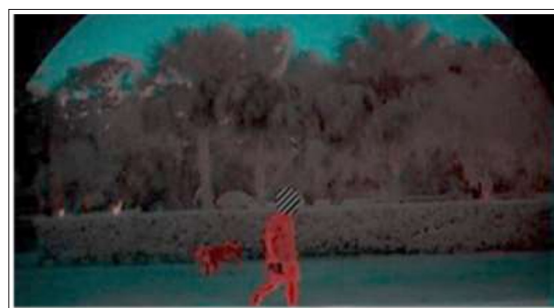
Figure 11: The Thermal Image was down Sampled to 128 \times 98 and then Interpolated Back to a High Resolution Before Fusion with the I 2 Image
