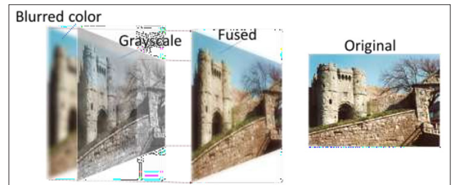
Figure 3: Blurred Color and Grayscale Images on the Left are Derived from the Original Image on the Right. The Fused Image is Obtained using Eq. 1
