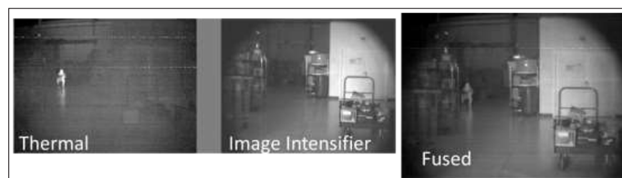
Figure 6: A Kneeling Person is Highlighted in the Thermal Image and Room Contents are Visible in the Reflected Image. The Fused Image Shows Both the Person and Room Contents
