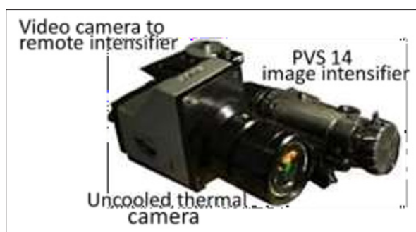
Figure 4: Reflective and Thermal Cameras used to Collect Most of the Fused Imagery
