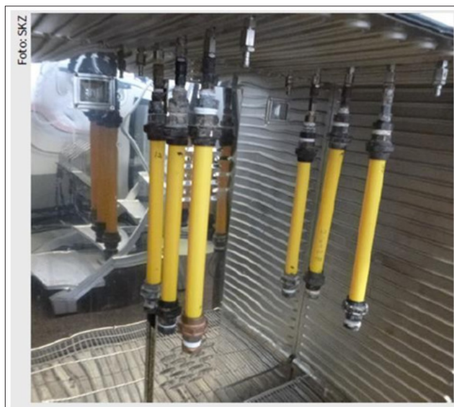
Figure 2: PA-U12 180 pipes in the test chamber for LTHS testing
