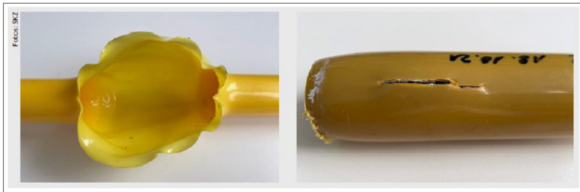
Figure 4: Examples of ductile (left) and brittle (right) failures of PA-U12 180 pipes from LTHS tests at 120° C
