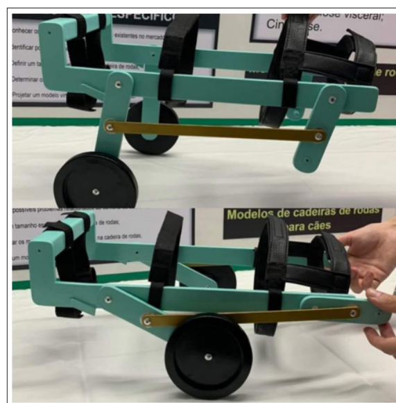
Figure 12: Wheelchair Model Manufactured with MDF Source: The author (2022).
