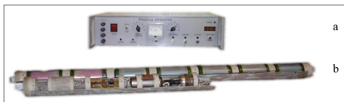
Figure 3: General View of the Device a. Control Unit b. Three-Phase Electromagnetic Vibro Exciter
