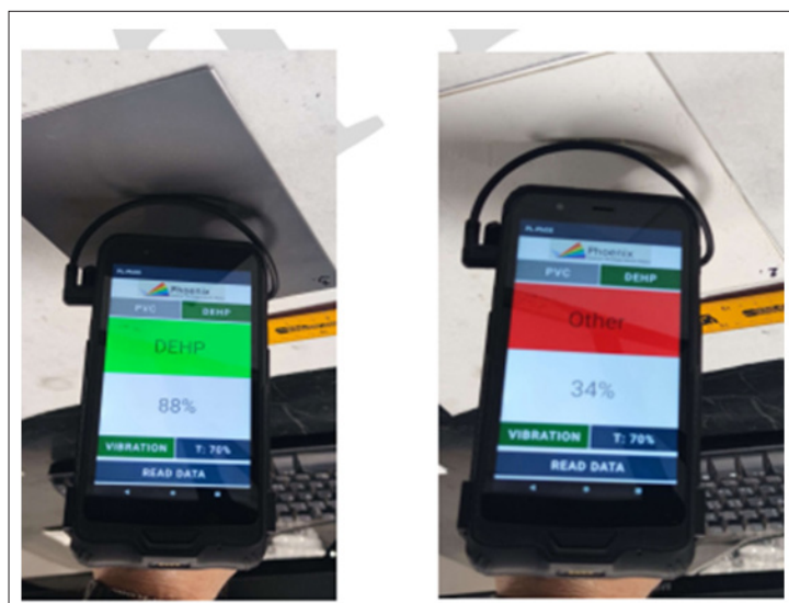
Figure 2: Detection Tests for the Presence of DEHP in PVC Products
