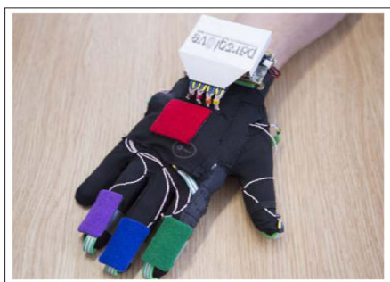
Figure 5: Parsglove Wearable Interface Designed to Capture Hand Ergonomics and Provide Interactive Input for Medical Palpation Training - taken from (Figure 1) [1].
