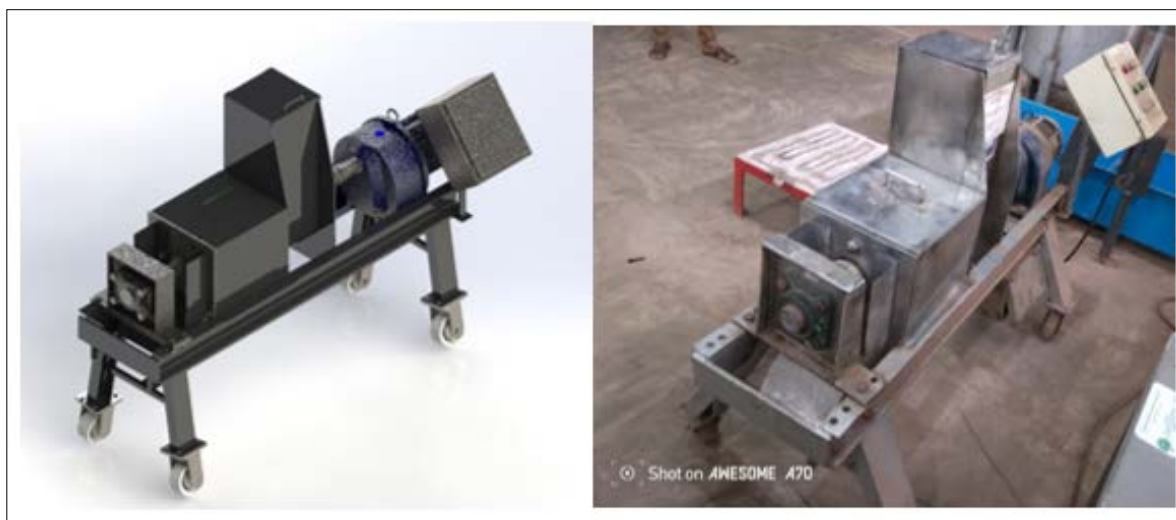
Figure 1: 3D CAD Model and Picture of the Virgin Coconut Oil Extraction Machine
