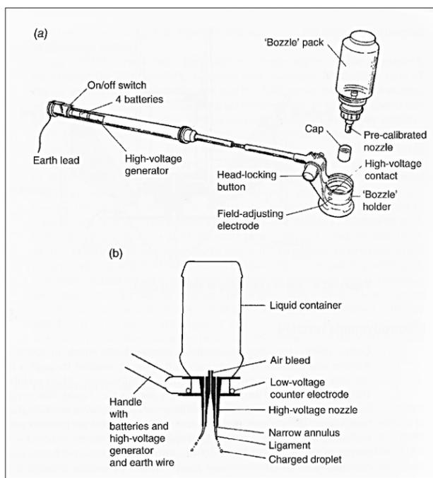
**Figure 10:** Diagrams Showing the Electrostatic Sprayer
