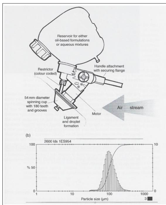
**Figure 8:** A hand-Carried Micron ULVA Sprayer with Rotary Atomiser
