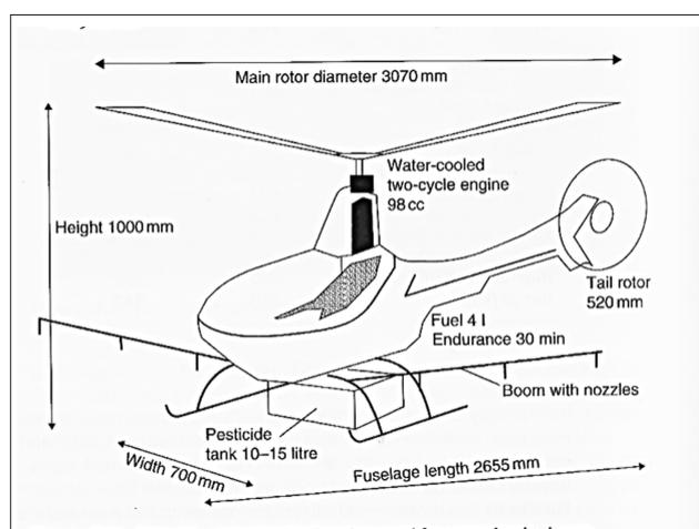
Figure 5: Unmanned Helicopter in Japan
