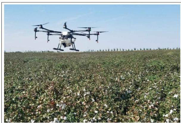
**Figure 6:** Drone Spraying Cotton in China
