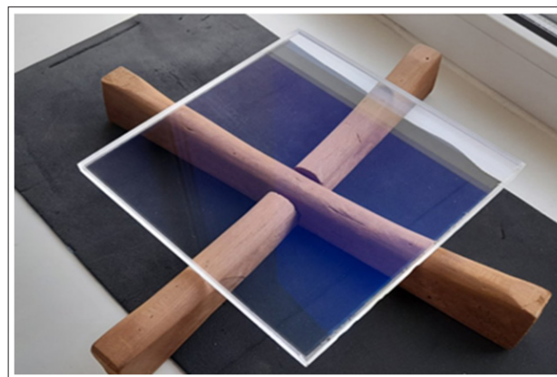
Figure 2: Photograph of a nonlinear optical element made from monocrystalline KDP crystal sized 180x180x10 mm.
