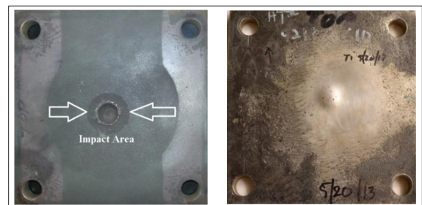
Figure 7: Visible damage on an A36 steel target on the Front sides (Left) and backside (Right).
