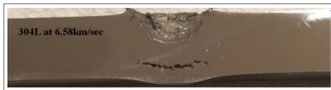
Figure 10: Crater zone in 304L targets subject at 6.58Km/s.
