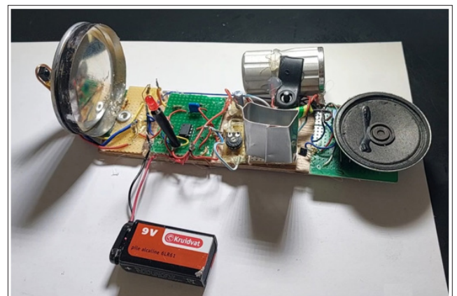
The image (4) is forming circuits inside the remote sensor device that sends and receives infrared rays.
