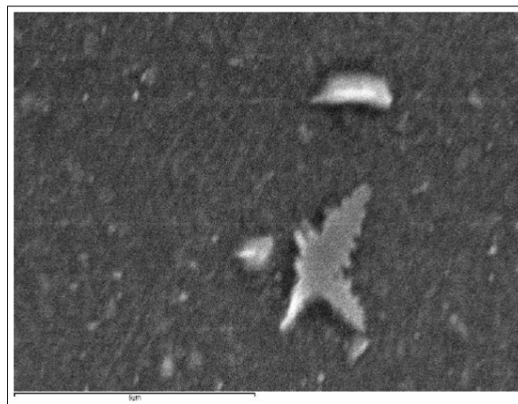
Figure 20: Microstructure, Obtained by Scanning Electron Microscopy, Showing a Stellate Iron Carbide inside the ARMCO Iron Grain
