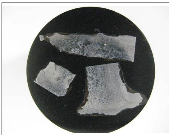
Figure 7: Macrograph of the examined, deep-drawn and metallographically prepared nail in Figure 6, with a clear metallic core, with a very heterogeneous microstructure of metallic grains
