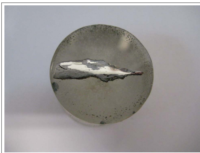
Figure 3: Macrograph of the nail under study, embedded and metallographically prepared, showing the iron core of the nail
