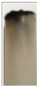
Figure 5: PVDF Sample after Burning Test
