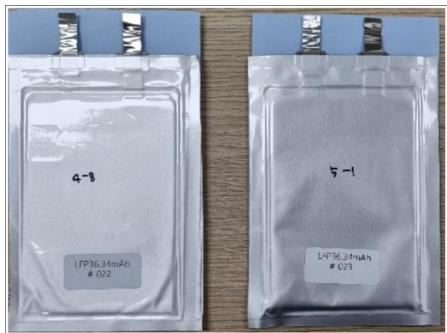
Figure 2: Normal Specimen (Left), Artificial Defect Specimen (Right)
