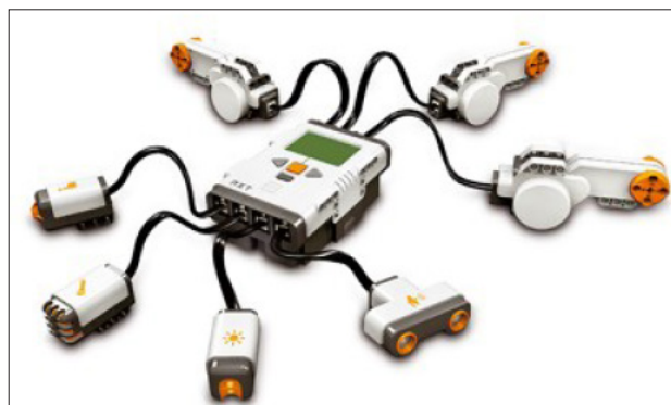
Figure 2: An Intelligent Cube with Connected Motors and Sensors
