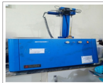
Figure 2: Automated Cloud and pour point analyzer (ASTM D250)
