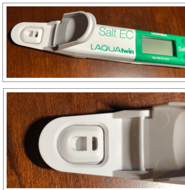
Figure S3: The compact salt meter (LAQUAtwin-salt-11 by Horiba) used in this research. It measures salt concentrations (0%–15%) with a relative precision of \pm 4\% , allowing direct measurement from a single drop.
