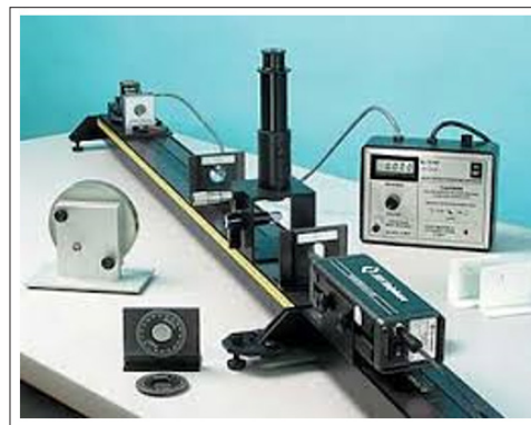
Figure 6: Modern laser interferometer for measuring the metric quantities [33].
