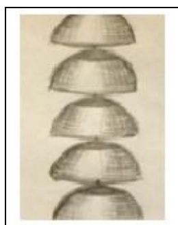
Fig. 11. A stack emitter made of hemispheres. If it is a 9 cm diameter “battery” consisting of nine hemispheres, then a power output is 4 watts.
