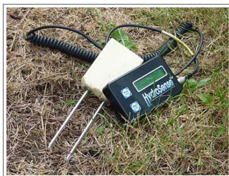
Figure 5: A Portable TDR Instrument for Measuring Soil Water Content (Photo by Maja Krzic, University of British Columbia, Vancouver Bc)
